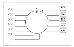
There is a choice of 7 power levels. The higher the power level, the more microwaves reach the food. When heating up food which cannot be stirred or turned during cooking, as with a plated meal, it is best to use a lower microwave power level.
